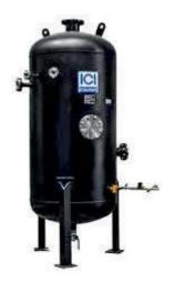
The BDV blowdown vessel has been designed to receive sludge that usually settle at the bottom of the steam boilers which is discharged during a bottom blowdown operation; this sludge is cooled and allowed to settle at the bottom of the tank before being discharged to the sewer thus limiting any risks for the operator and damage to the environment. The blowdown vessel complies with the PED Directive 2014/68/EU Provided with:
